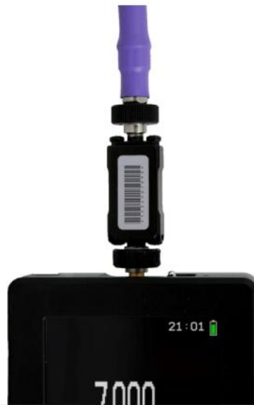
SG Compact interconnected with low pass filter P/N J0ALPF09
